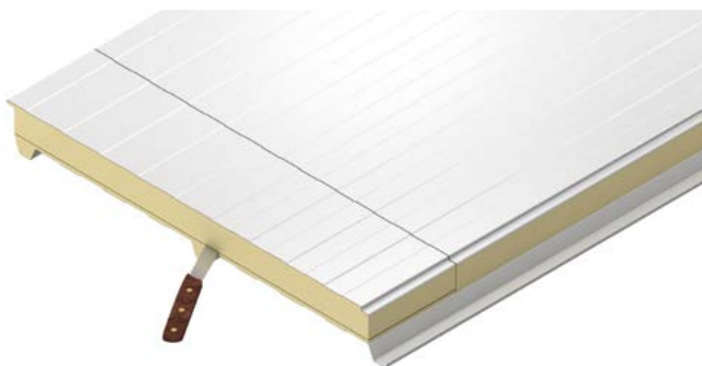
Using the same knife, cut along the bottom edge of the foam
