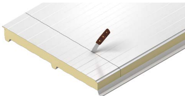
Using a serrated knife, cut through the foam
