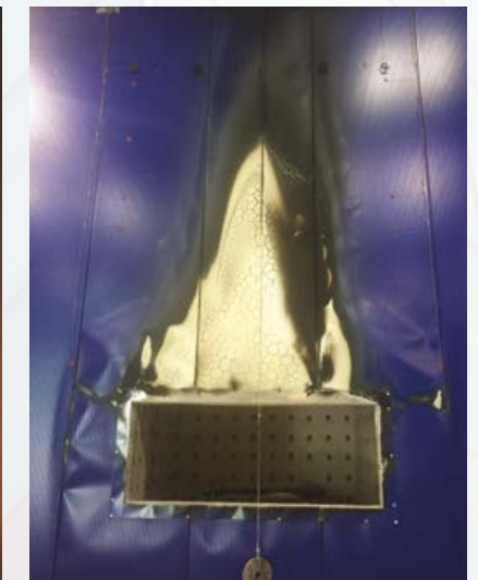
End of test showing the insulated panel system does not contribute to fire spread.
