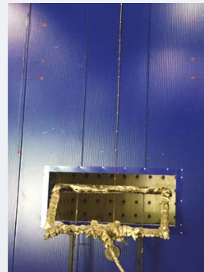
Test set up – Kingspan insulated panels installed in a full scale NFPA 285 test.
