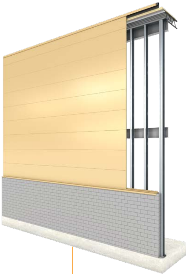
Insulated Metal Wall System with CMU Blockwork
