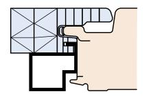
Wall light panel KS1000 WL is a product designed for any buildings where wall panels Kingspan KS1000 AWP are used. The panel is made from polycarbonate and it helps to reach optimal thermal values of the insulated building. The panel is suitable for all types of buildings except those with high air humidity caused by the influence of building users or production processes. They are also not suitable for buildings with low inside temperature.
