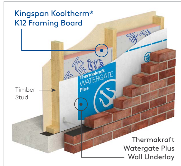
Figure 6. Kooltherm K12 Framing Board fitted between timber wall studs.
