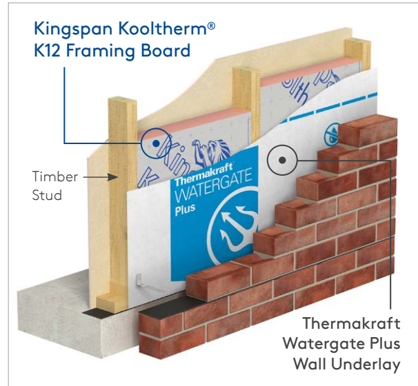
Figure 4. Timber Frame Construction with Insulation between Studs.
