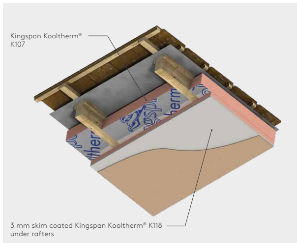
Figure 8: Mechanically fixed to timber rafters with Kingspan Kooltherm® K107 Pitched Roof Board between rafters
