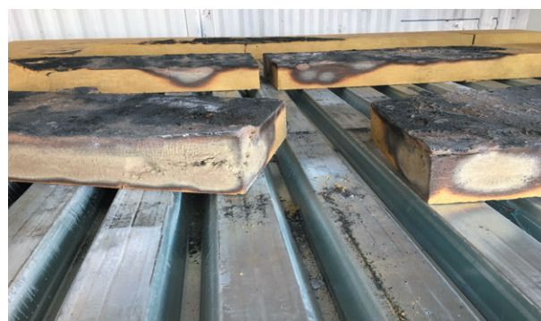
rock mineral fibre boards that had been stored outside, and temperatures up to 760°C were recorded.
